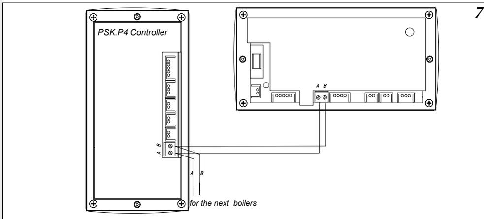
Fig.7 Additional electrical connection for boilers in cascade
