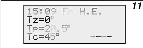
Fig.11 Main view in configuration – CH „off” and DHW „on”
