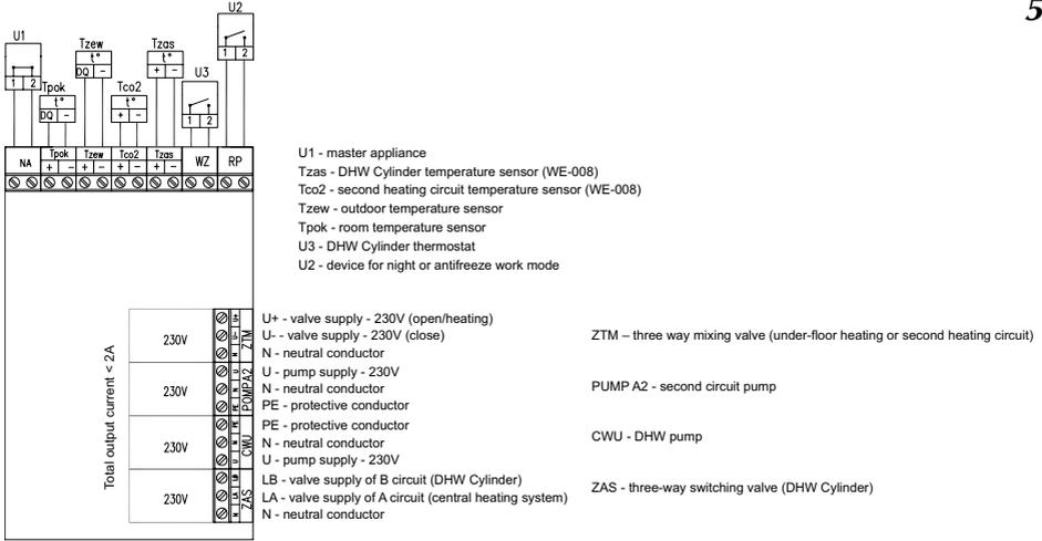
Fig.5 Connecting external appliances to the ZIO board
