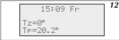
Fig.12 Main view in configuration – central heating mode „off” and DHW mode „off”
